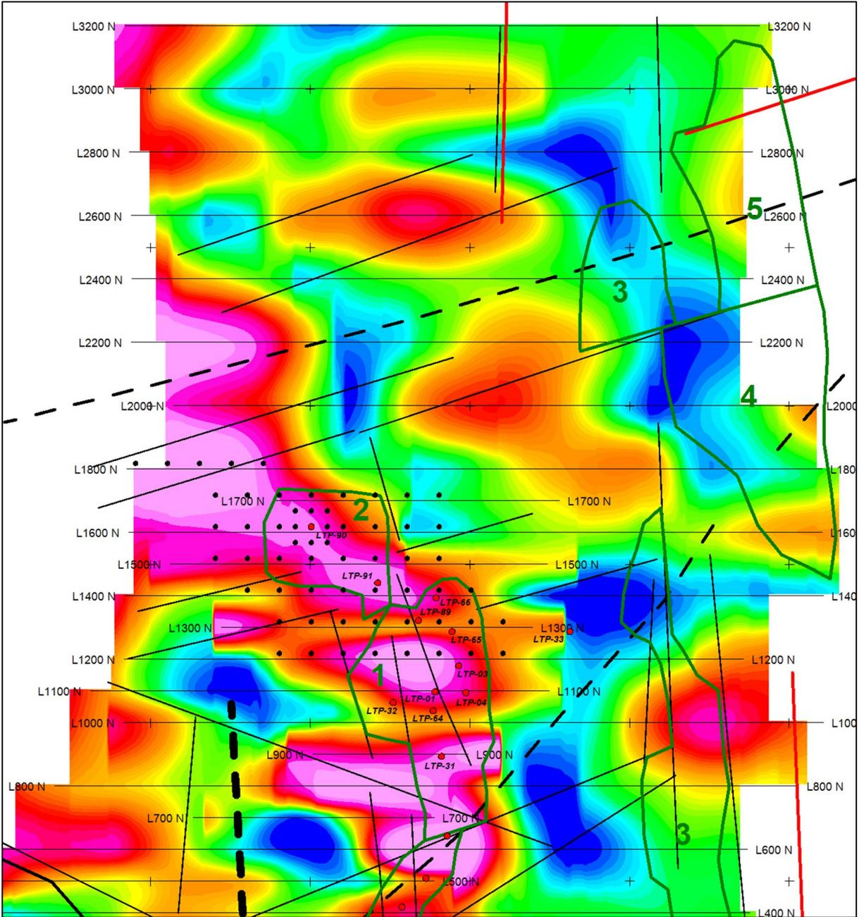
Figure 4. Conductivity 283m below ground (Zone 2N), with existing and proposed drillholes.
