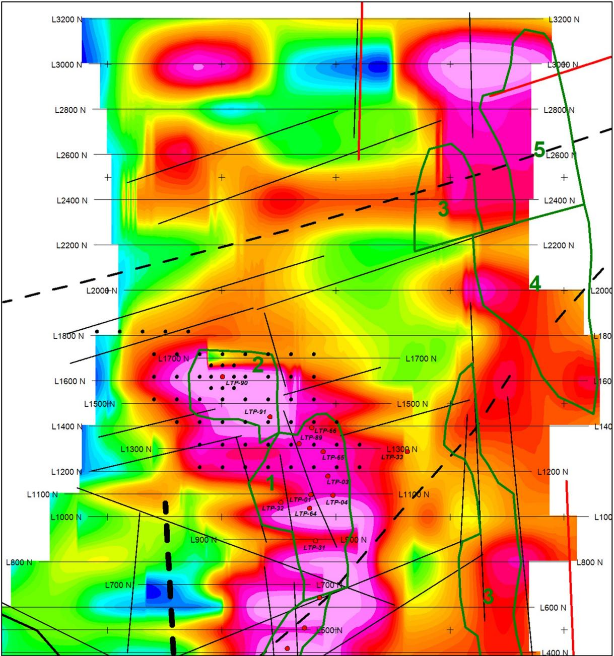
Figure 3. Chargeability 283m below ground (Zone 2N), with existing and proposed drillholes.
