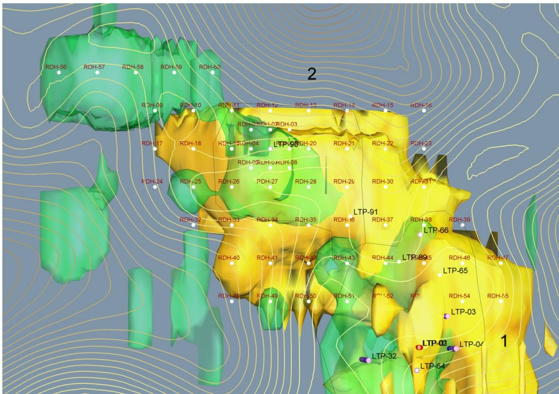
Figure 10. Existing and proposed drillholes from above, showing conductivity and chargeability.
