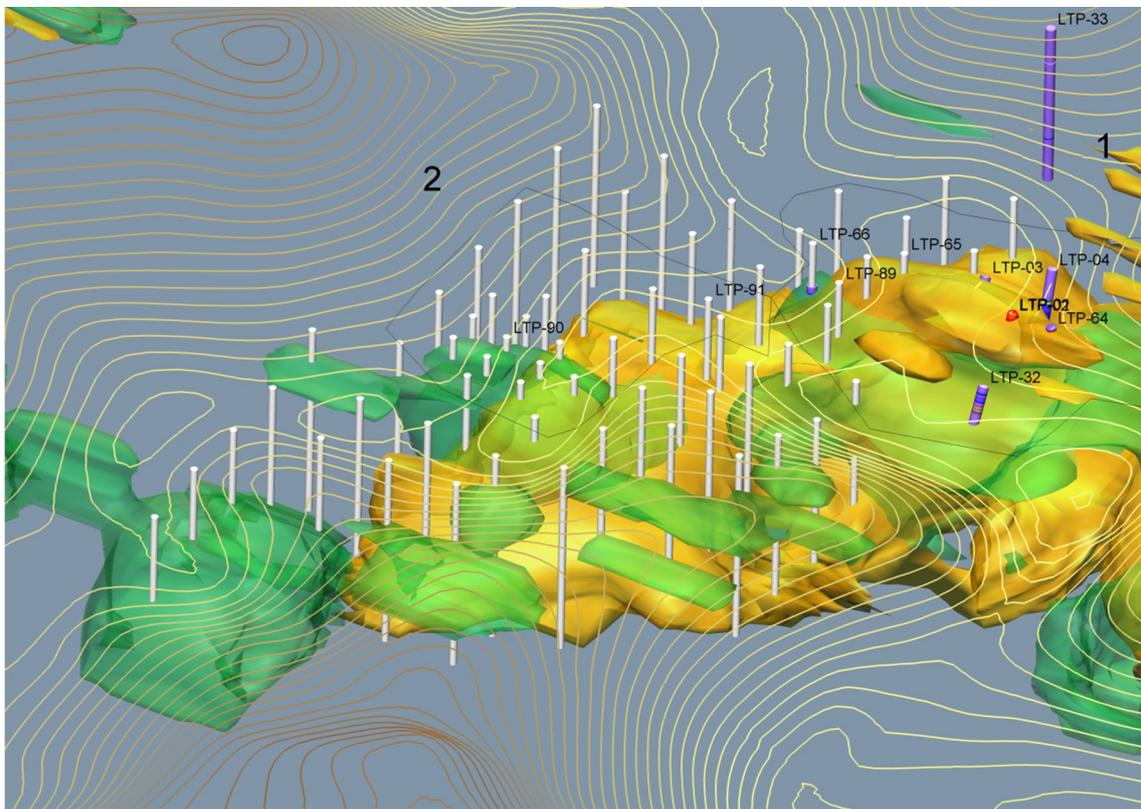
Figure 11. 3D view of existing and proposed drillholes.
